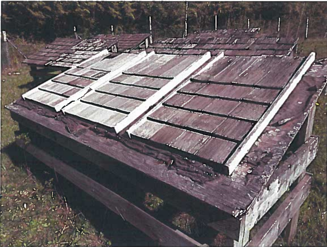
Figure 10. Western redcedar shingles dip treated with DDACarbonate and alkylamine oxide (left), pressure treated with DDACarbonate and alkylamine oxide (centre), and untreated (right).
