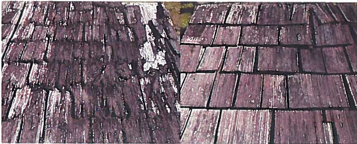
Figure 1. Untreated western redcedar shakes (left) and CCA-B treated western redcedar shakes (right) after 45 years of exposure in Maple Ridge, British Columbia.
